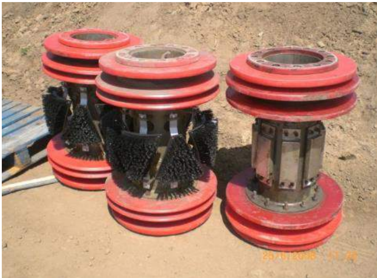
Figure 3-27: Variety of Cleaning Pigs (Brushes and Magnetic)
